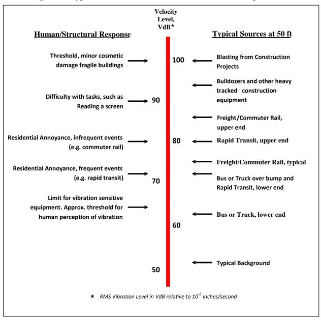
Figure 1-2 Typical Vibration Levels and Human/Structural Responses
