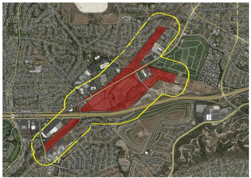
Figure 4-2 80 dBA L<sub>eq</sub>(8-hr) Contour For Helicopter Use in ROW
