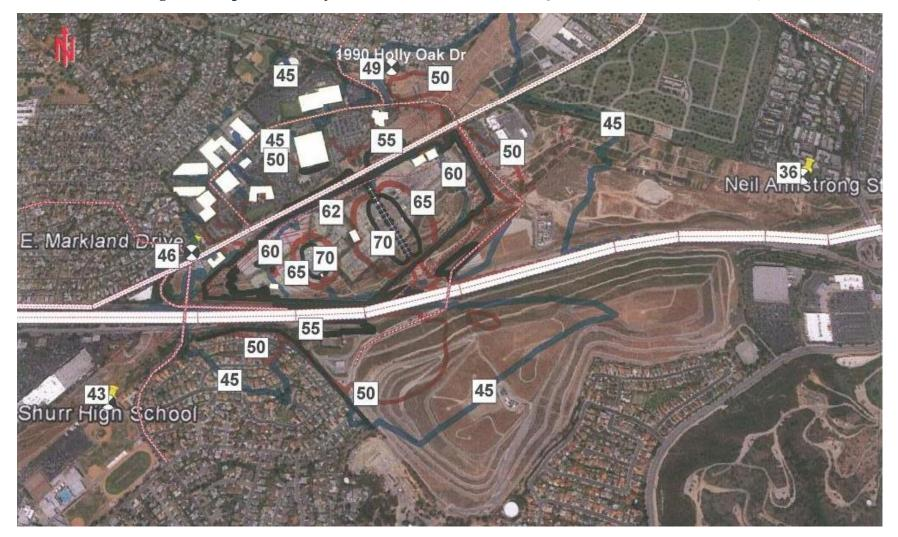
Figure 5-2 Operational Leq Noise Contours with 4 decibel Quieter Bank AA Transformers, dBA
