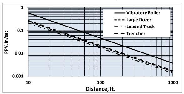
**Figure 4-6 Construction Vibration Amplitudes**
