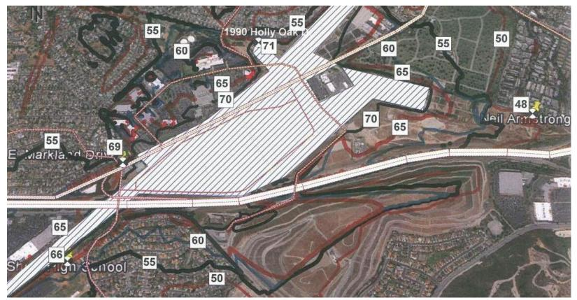
Figure 4-1 Construction Noise Contours – L<sub>eq</sub>(8-hr), dBA
